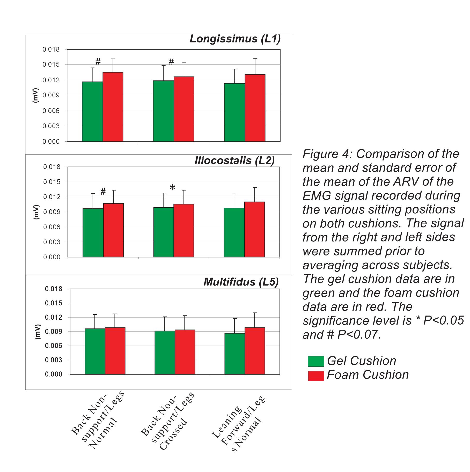
Preliminary results indicate that when subjects are seated with no back support, the lower back muscles are less active with the gel cushion than with the foam cushion. (The unsupported back position is the normal sitting position). One possible explanation is that the greater conformity of the gel cushion provides a more stable support for the pelvis which, in turn, requires less activity from the back muscles for stability
