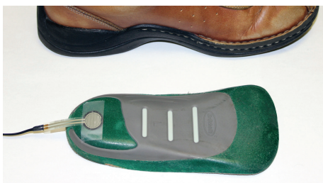
Figure 12. Affixing the FSR membrane to the bottom of the inner sole.
