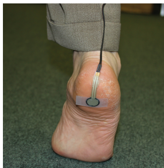
Figure 10. Affixing the FSR membrane directly on the heel.
