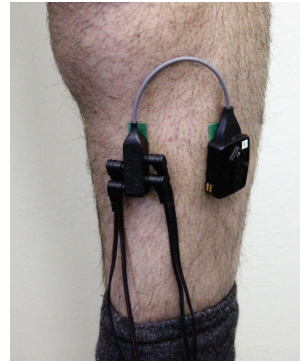
Figure 15. Placing the FSR Sensor on the body.
