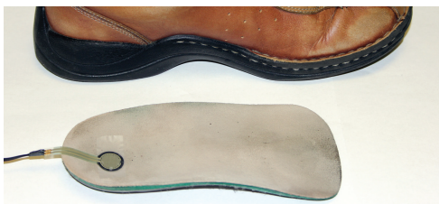
Figure 11. Affixing the FSR membrane to the top of the inner sole.
